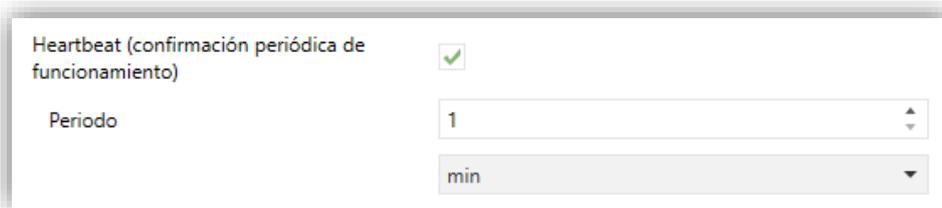
The screenshot shows a configuration window for the 'Heartbeat (confirmación periódica de funcionamiento)' parameter. It features a green checkmark icon indicating it is enabled. Below this, there is a 'Periodo' field with a dropdown menu showing the value '1' and a unit dropdown menu showing 'min'.
